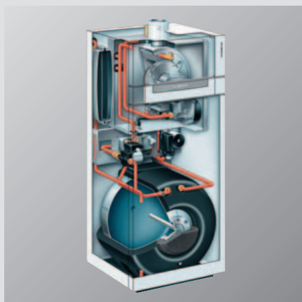
Vitodens 333-F 3,8 do 26,0 kW z integriranim hranilnikom (prostornina 86 l)
